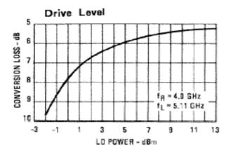
Drive Level: The maximum recommended drive level is +13 dBm.
