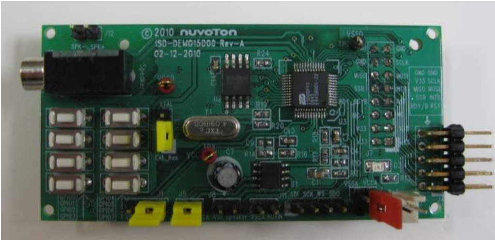
Figure 1 – Top view of ISD-DEMO15D00 Rev-A board
