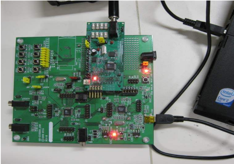
Figure 6 – ISD15D00 is connected onto ISD-ES15D00_USB mother board
