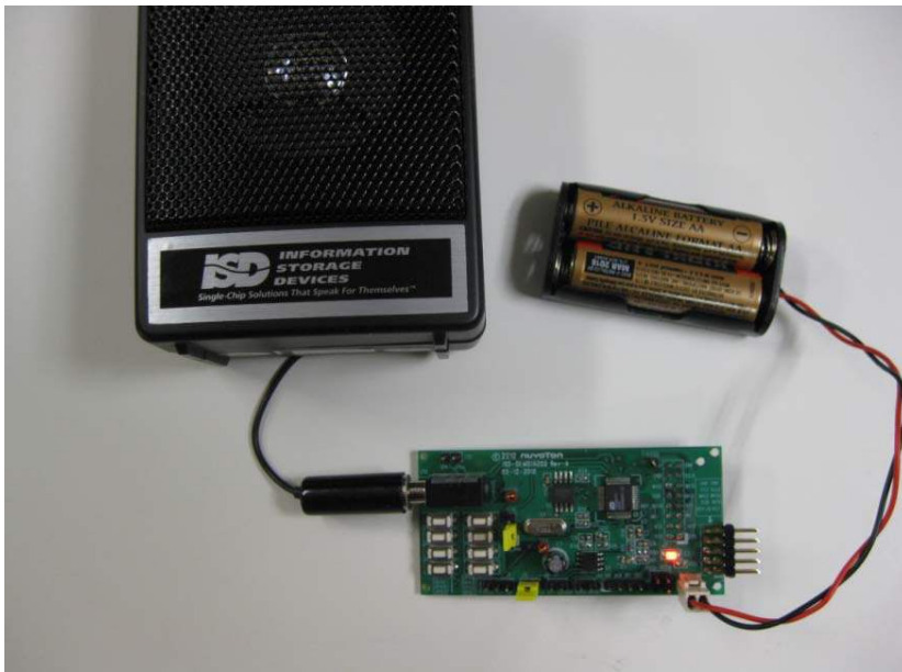
Figure 8 – ISD15D00 demo board standalone evaluation.
