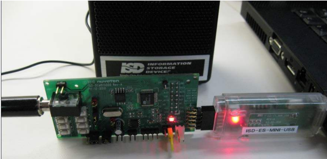
Figure 4 – A complete evaluation environment for ISD15D00 device
