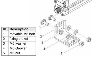
Note: Shipment contains different quantity of brackets, depending on the length of the SLC. Longer SLC contains a higher number of brackets, following the rule of every 400 mm one bracket.
