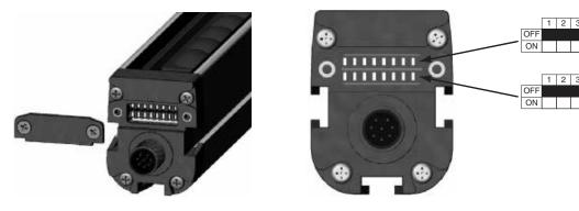
Note: There are two lines of dip switches in each transmitter and receiver. The settings must be done for both lines. Change the setting of the dip-switch and close the cap again. The light curtain can now be reconnected to the power supply.
