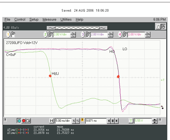
Figure 31. V_{LO} and V_{HO} Falling Edge Delay Matching
