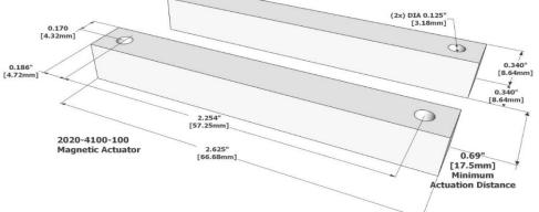
All measurements are in Inches [millimeters]
