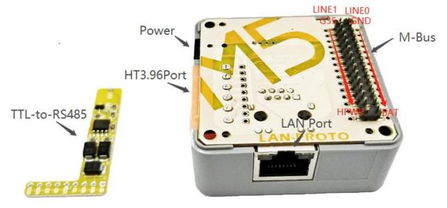
**The figure below tells you how the TTL-to-RS485 adapter board connected onto LAN backplane** *The serial port pins on the RS485 board will be connected to the GPI016 and GPI017 of the LAN backplane.*
