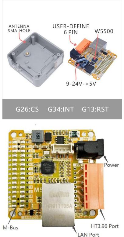
If you need to add RS485 interface, soldering the RS485 board onto the mian board pin correspondingly.
