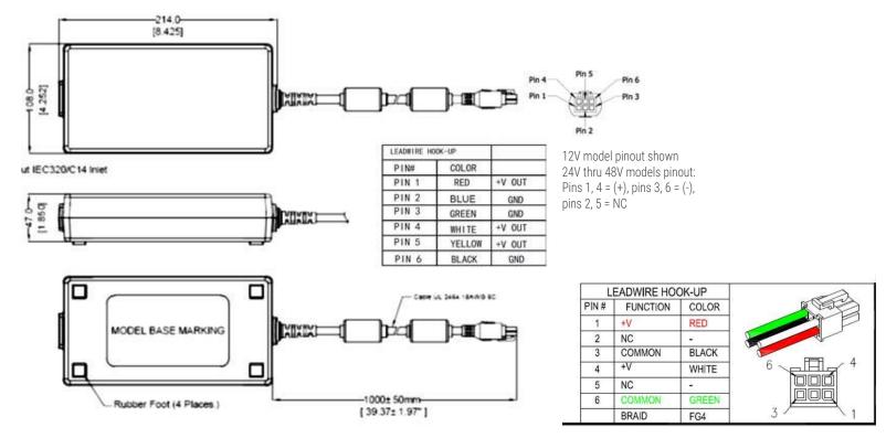
Note: Pins 4,5,6 are located closest to the locking tab
