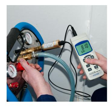
PCE-932 is an easy-to-use, digital, handheld device for high pressure measurement in hydraulic and compressor systems, pumps, tanks and silos in chemical, manufacturing, plastics and HVAC industries. This portable pressure measuring device can be connected to pressure sensors with ranges up to 400 bar (each with a 1.2 m connecting cable).
