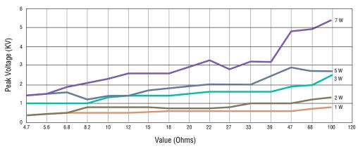
1.2/50  $\mu s$  Peak Voltage Limit (10 pulses at 10 sec. intervals,  $\Delta R < 5$  %)
