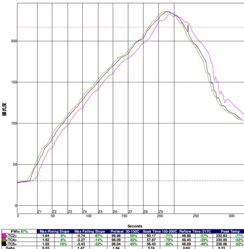
Figure 7 - Example solder reflow profile (AMW037-E03 evaluation board)
