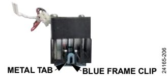
Figure 6. Heat Sink Installation Step 1
