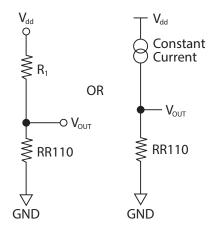
RR110 Magnetoresistance Application Circuit
