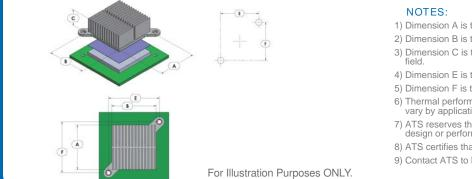
1) Dimension A is the length of the heat sink in the direction of the flow.
