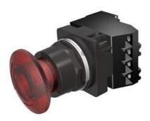
30mm BlackMax, Epoxy Coated Corrosion Resistant Complete Metal Unit Illuminated Twist-to-Release Transformer type, 480V AC Incandescent Lamp Mushroom Head Cap Small 1.79" (45 mm) Plastic Cap, Red 2 Position Maintained, Twist-to-Release with 1 N.O. - 1 N.C. Heavy Duty Contacts, A600/P600 UL Listed, CSA Certified NEMA 1,3,3R,4,4X,12,13 & Automotive Standards
