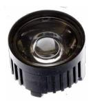
These water-clear polycarbonate lenses with black holders are specifically designed to mate with Optek's 6x6mm power surface mount LEDs (OVSxxxCR4 Series) to provide a more narrow beam angle. Lenses are available in both 15° and 23° viewing angles. The lenses and holders sit firmly over the LED component and is easily attached to the PCB/MCPCB with adhesive.
