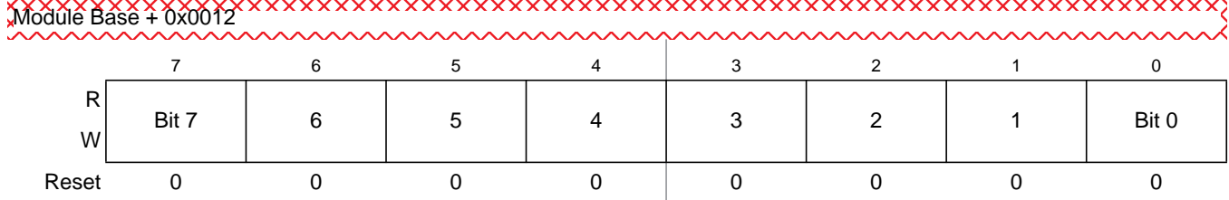
Figure 10-21. PWM Channel Period Registers (PWMPER0)
