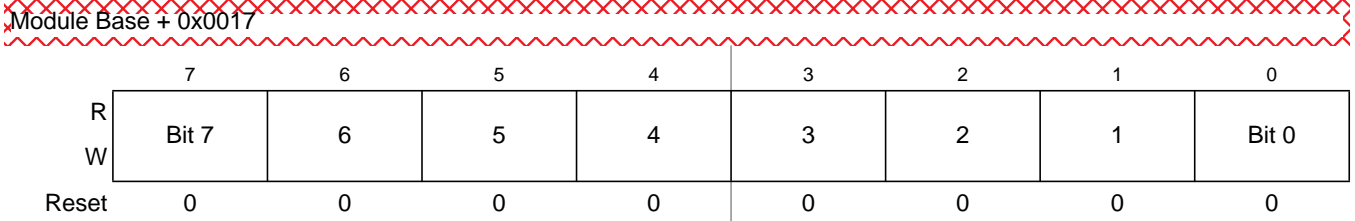
Figure 10-26. PWM Channel Period Registers (PWMPER5)
