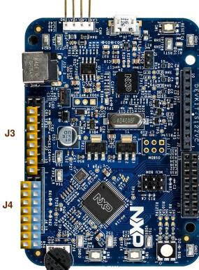
Arduino Compatibility The internal rows of the I/O headers on the DEVKIT-S12VC are arranged to fulfill Arduino<sup>™</sup> shields compatibility
