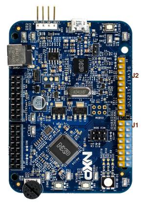
Arduino Compatibility The internal rows of the I/O headers on the DEVKIT-S12ZVC are arranged to fulfill Arduino<sup>™</sup> shields compatibility
