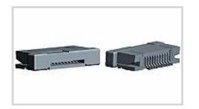
Connector System: Flex-to-Board Number of Positions: 23 Centerline (Pitch): .5 mm [ .02 in ] Insertion Force Type: Zero Insertion Force (ZIF) PCB Mount Orientation: Right Angle
