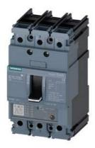
circuit breaker 3VA5 UL frame 125 3-pole, starter protection TM120M, AM, In=5A without overload protection short-circuit protection Ii=3...7 x In nut keeper kit on both sides
