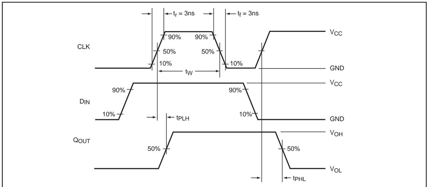
Figure 3. AC Waveforms
