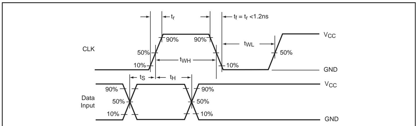
Figure 4. AC Waveforms
