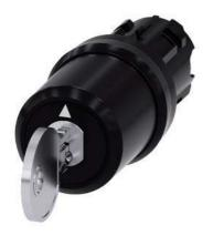
Key-operated switch BKS, 22 mm, round, plastic, lock number S1, with 2 keys, 3 switch positions I-O-II, latching, actuating angle 2x45°, 10:30h/12h/13:30h, Key removal II, with laser labeling, upper case and lower case, always upper case at the beginning of the word
