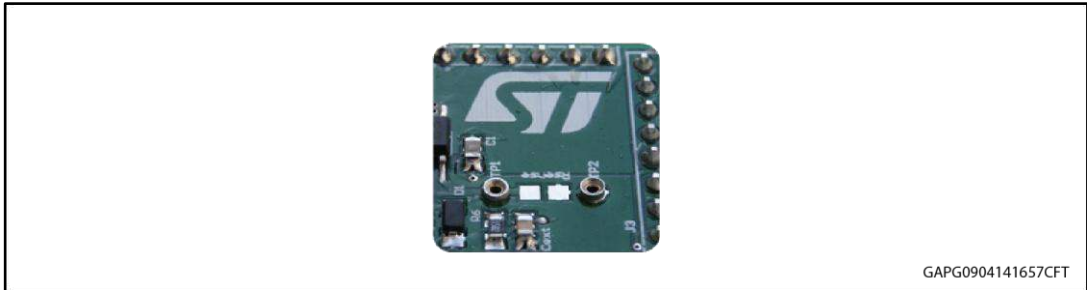
Figure 4: Mounting through-hole sense resistor
