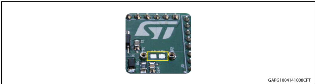
Figure 5: Pads for soldering SMD resistor
