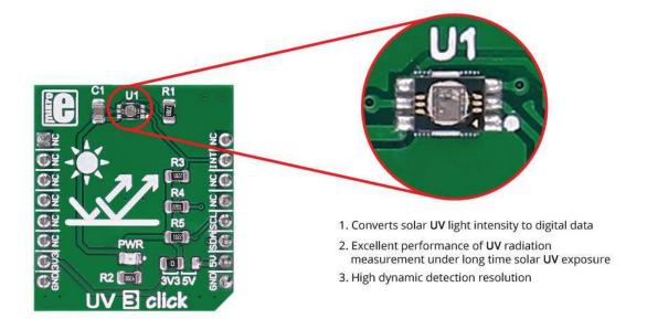
VEML6070 incorporates a photodiode, amplifiers, and analog/digital circuits into a single chip. VEML6070's adoption of Filtron<sup>TM</sup> UV technology provides the best spectral sensitivity to cover UV spectrum sensing. It has an excellent temperature compensation and a robust refresh rate setting that does not use an external RC low pass filter. VEML6070 has linear sensitivity to solar UV light and is easily adjusted by an external resistor.
