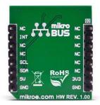
**UV 3 click** is an advanced ultraviolet (UV) light sensor with I2C protocol interface. The click carries VEML6070 UVA light sensor designed by the CMOS process. UV 3 click runs on either 3.3V or 5V power supply.
