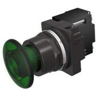
30mm BlackMax, Epoxy Coated Corrosion Resistant Complete Metal Unit Illuminated Push-Pull Operator Transformer type, 480V AC Incandescent Lamp Mushroom Head Cap Small 1 3/4" (44.5 mm) Plastic, Green 3 Position Pull-Momentary/Push-Maintained UL Listed, CSA Certified NEMA 1,3,3R,4,4X,12,13 & Automotive Standards
