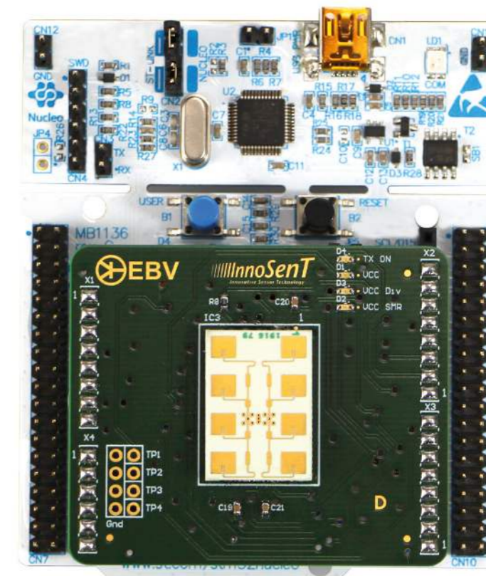
Figure 3: SMR-board and STM32 board connection
