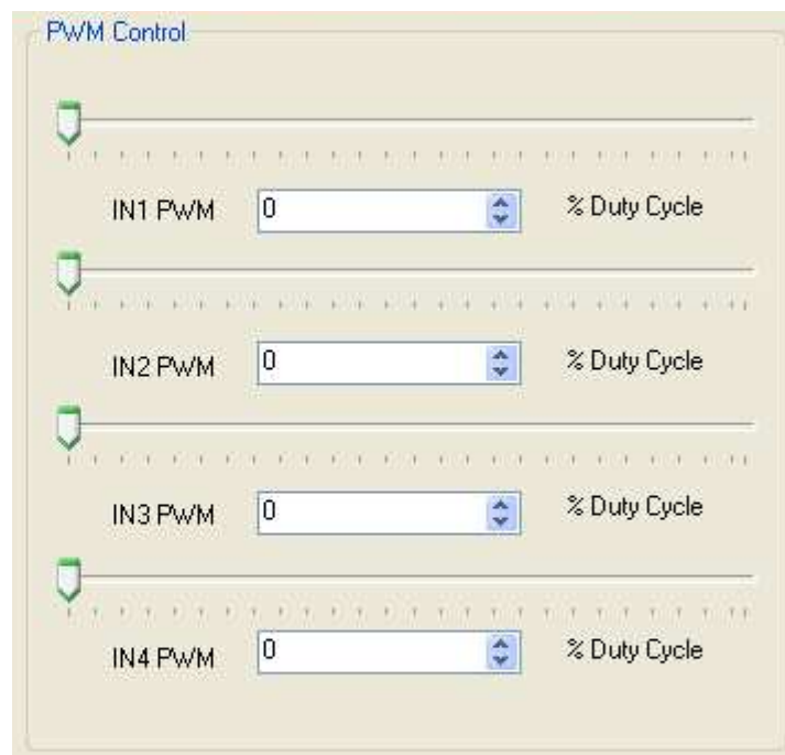
Figure 4. DRV8844 PWM Control Window
