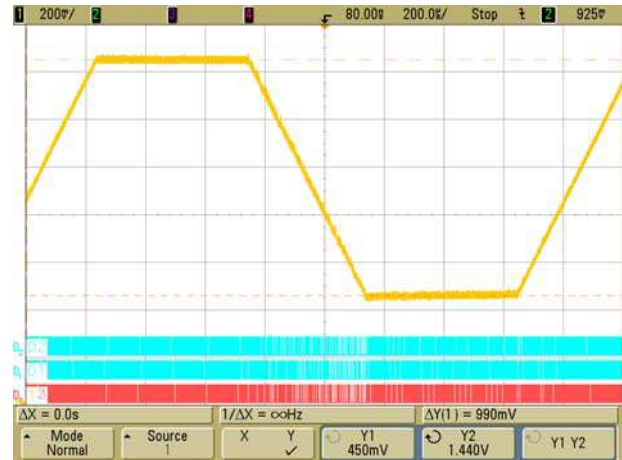
Figure 6. DVID Waveform (by VTT, 0.5 V-1.5V) 1-Vo D0~D2-PWM1~3
