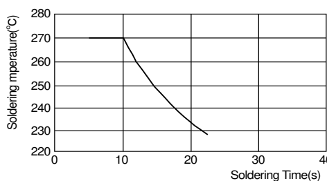
[Allowable Flow Soldering Temperature and Time]
