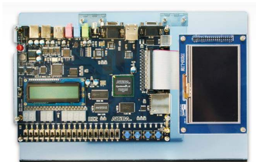
Figure 1.3 Connect the other end of IDE cable to the DE2 board's expansion port (innermost expansion port)
