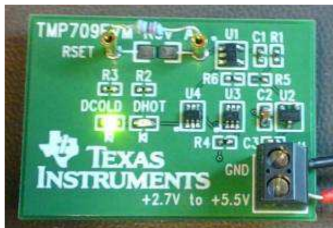
Figure 4. On-Board LEDs Indicating that Current Temperature is Below the Limit Set by Rset
