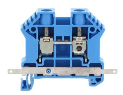
Feed-through terminal, Screw connection, Mounting type: Mounting rail TS 35/7.5, Rated cross-section: 16 mm², Width: 10 mm, Colour: Blue
