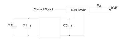
C1/C2 100uF/35V (Low internal resistance capacitance)
