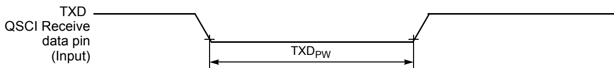
Figure 10-13 TXD Pulse Width
