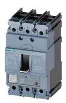
circuit breaker 3VA5 UL frame 125 breaking capacity class S 25kA @ 480 V 3-pole, line protection TM230, FTAM, In=30A overload protection Ir=30A fixed short-circuit protection li=5...10 x In cable connection on both sides
