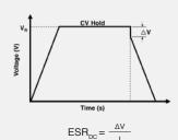
$\label{eq:condition} \mbox{where C is the capacitance (F);} \\ \mbox{I is the absolute value of the discharge current (A);}$
