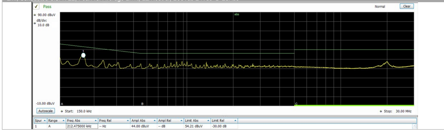
EMI; Conducted CISPR 22; Peak vs. Average Limit; L2/Neutral; 208Vac 24Vdc @ 25A
