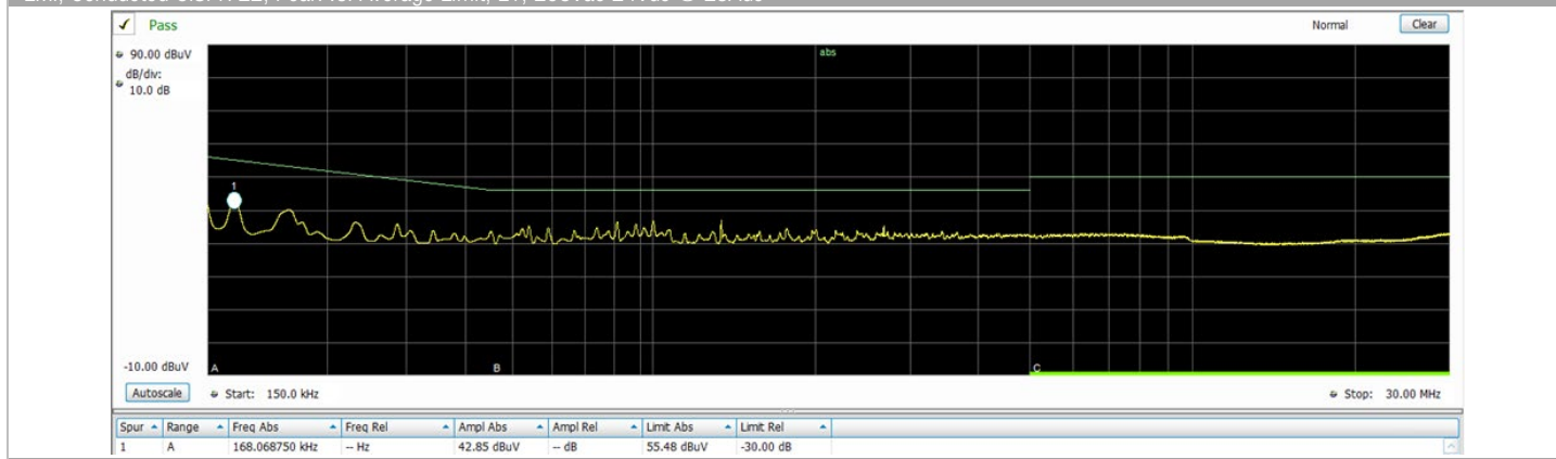
EMI; Conducted CISPR 22; Peak vs. Average Limit; L2/Neutral; 208Vac 24Vdc @ 25A
