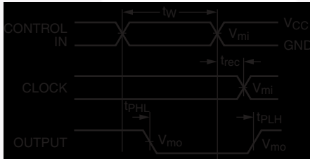
Propagation Delay, Pulse Width and t_{rec} Waveforms
