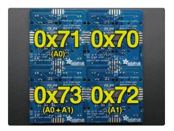
When setting the board addresses (by bridging the solder points on the back), use the values shown here.
