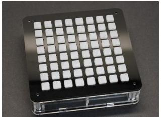
Install the clear top "waffle" piece. Since you'll still be holding the Trellis down, start from one edge, aligning the notches with the tabs on the side pieces, and swing this down into place as you remove your other hand.
