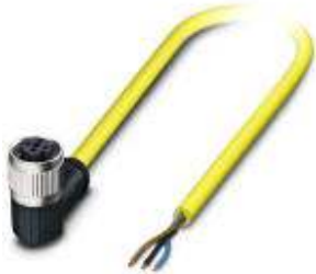
Sensor/Actuator cable, 3-position, TPE, yellow RAL 1021, free cable end, on Socket angled M12 SPEEDCON, A-coded, Cable length: 5 m
