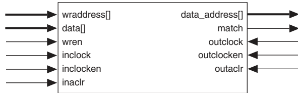
Figure 23. APEX 20KC CAM Block Diagram
