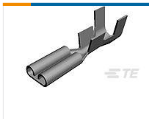
TE Part #160484-4 110 FASTON,REC.,20-17 AWG,BR
