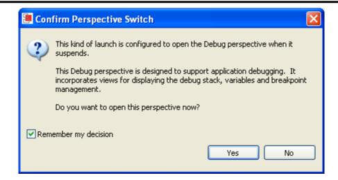
5. The Red Suite debugger automatically connects to your evaluation board, programs the flash, and runs to the beginning of the main () function. From here, you can examine and modify memory, program variables and processor registers, set breakpoints, step, and other typical debugging activities. To run the program, select "Resume" from the Run menu.
