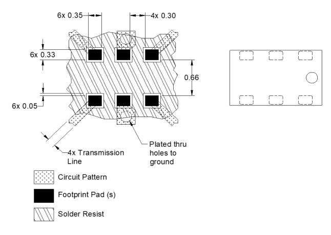
Dimensions are in Millimeters Mounting Footprint
