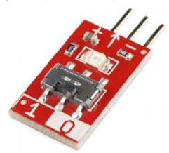
Each Input Block has a two-position switch, which you'll use to set the block as either 1 or 0 (TRUE or FALSE, ON or OFF).
