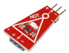
You can connect either an **Input Block** or the output from another **Gate Block** to this input. This male connector can be plugged into either the input of another gate or a **Power Block**.
