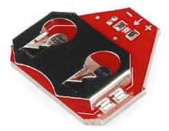
The Power Block runs on a single **20mm coin cell battery**, which optimally provides around 3V, and should last for quite a while. The LogicBlocks can work at voltages between 2 and 5V, and they consume very little current.
