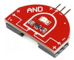
You can connect either an **Input Block** or the output from another **Gate Block** to these inputs. The male output header can be plugged into either the input of another gate or a **Power Block**.
