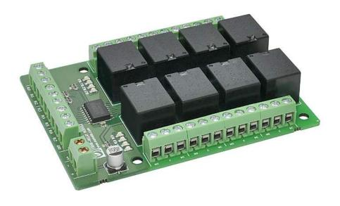
8 Channel Relay Controller Board User Guide
