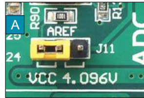
Figure 7-4: The position of jumper J11
