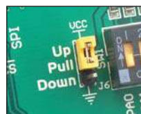
Figure 13-3: J2 in pull-up position
