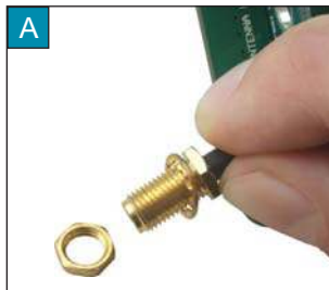
Figure 9-4: Screwing cable into antenna holder
