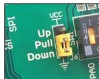
Figure 13-2: J2 in pull-down position
