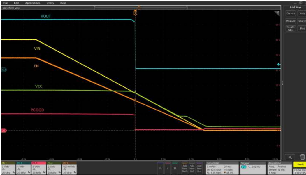
Figure 5 Shutdown with Enable de-assertion at 4A load (Ch1:PV IN , Ch2: V OUT , Ch3: PGood, Ch4:V CO , Ch5: Enable)
