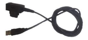
Communication:Bi-DirectionalBaud Rate:9600Data Bit:8Stop Bit:1Flow Control:None
