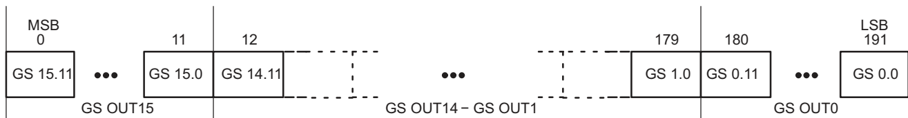
Figure 17. Grayscale Data Packet Format
