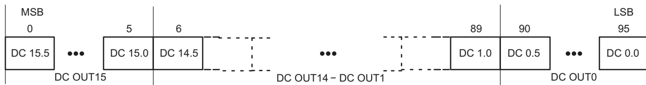
Figure 15. Dot Correction Data Packet Format
