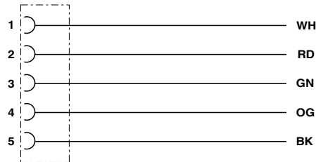
Contact assignment of 7/8" plugs/sockets, cable type 410
